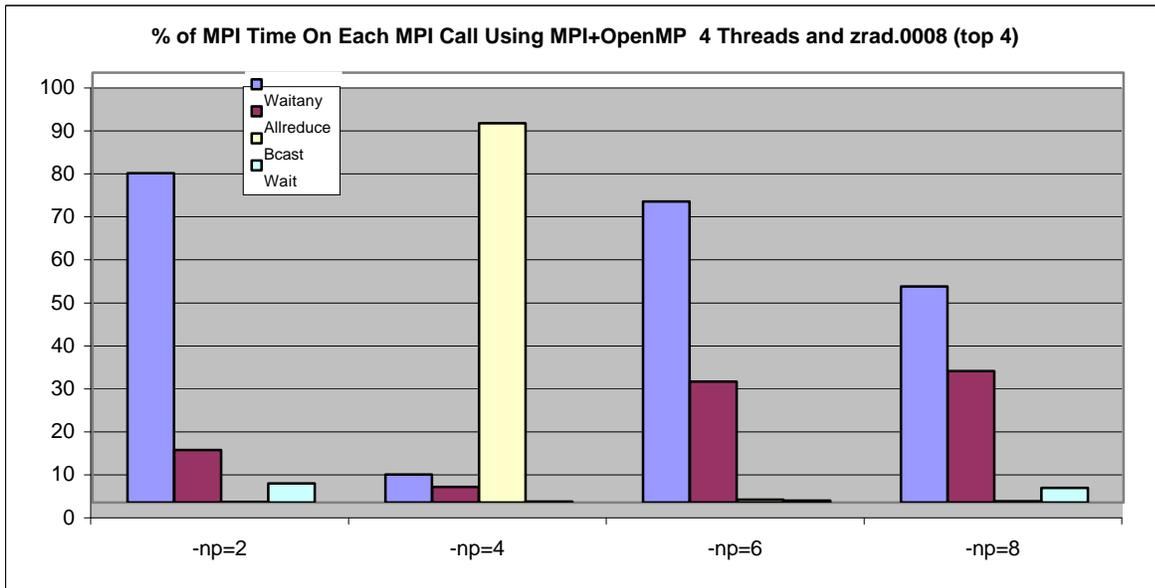
\* Compare to MPI/OpenMP with 2 threads; in MPI/OpenMP with 4 threads MPI calls does not show any major change. Increasing number of OpenMP threads does not lead to any change MPI time.
