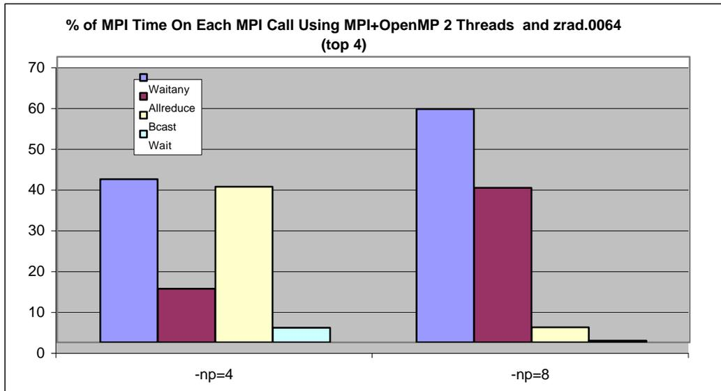
\* When increasing input size, it likely needs to increase the number of nodes. In the case of "np=2", "Waitany", "Allreduce" and "Bcast" takes longer than "Waitany" in the case of "-np=8". When the number of nodes is small, there is likely a lot of communication between nodes and also facing the problem of call blocking and synchronization.
