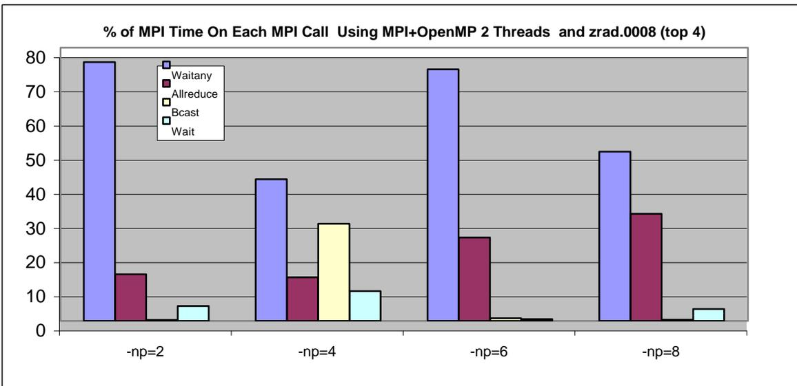
\* MPI/OpenMP reduces significantly MPI time, when distributes multiple blocks to each single node. The communication among processes within a node is faster then communication among processes between nodes.
