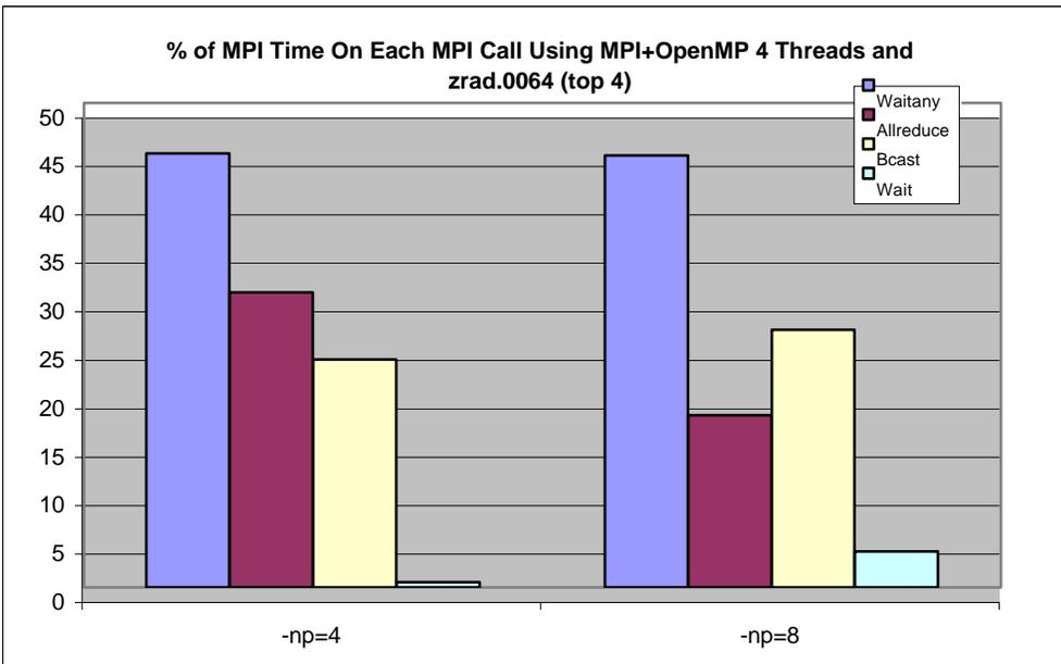
\* Compare to MPI/OpenMP with 2 threads; in MPI/OpenMP with 4 threads MPI calls does not show any major change. Increasing number of OpenMP threads does not lead to any change MPI time.
