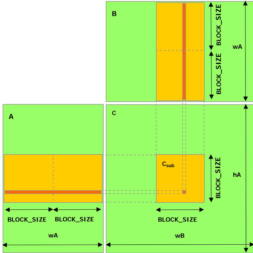
Each thread block computes one sub-matrix  $C_{sub}$  of C. Each thread within the block computes one element of  $C_{sub}$ .
