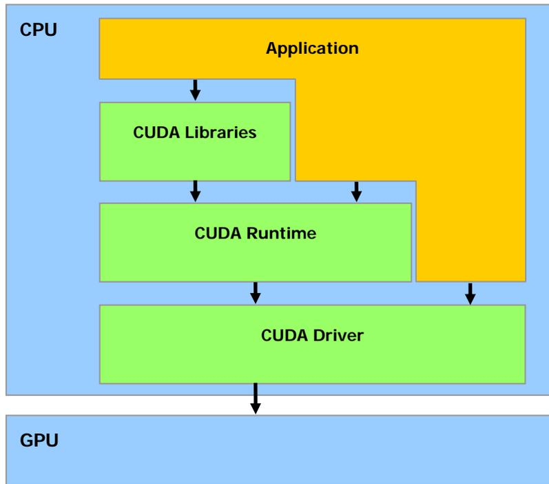
Figure 1-3. Compute Unified Device Architecture Software Stack
