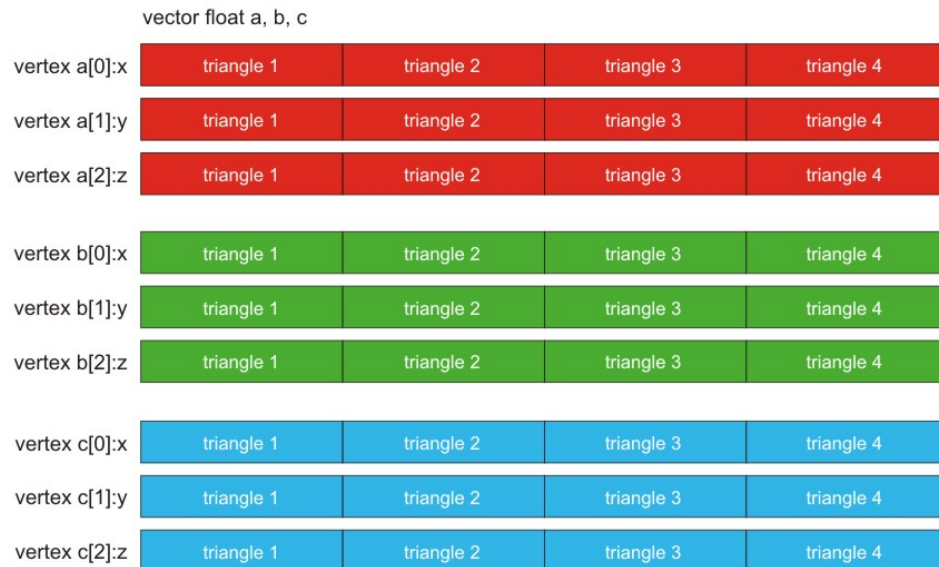
Figure 25. Structure-of-arrays data organization for four triangles
