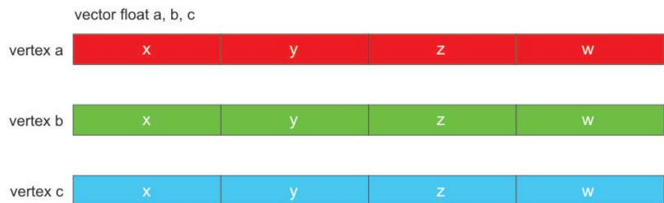
Figure 24. Array-of-structures data organization for one triangle
