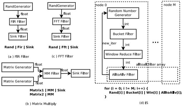
Figure 8. Filter Structure for Benchmarks
