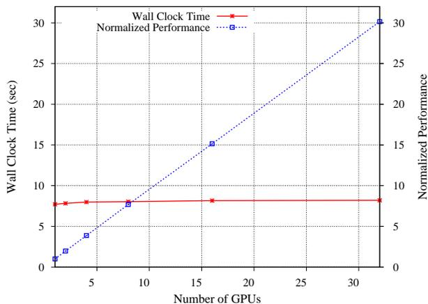
Figure 11. Weak Scaling in 3D Stencil on up to 32 GPUs
