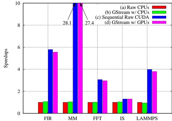
Figure 9. Speedup of Benchmarks on 32 CPU/GPU Nodes
