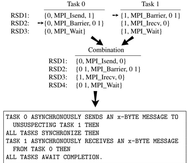
**Figure 4: Operation of Algorithm 1**
