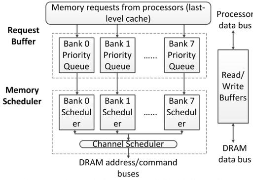
Fig. 4. Logical Structure of DRAM Controller
