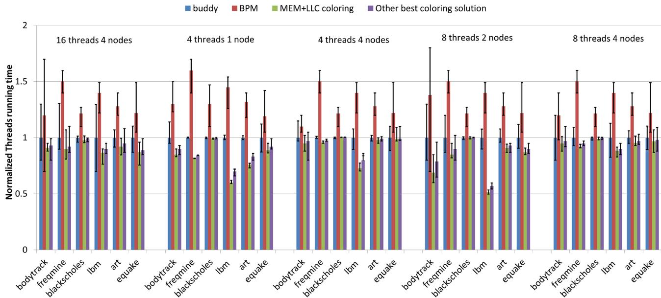
Fig. 13. Threads running time
