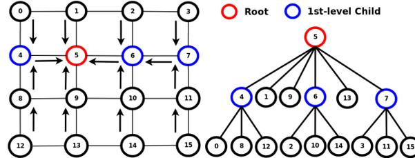
Fig. 5: Reduction Tree: Setup
