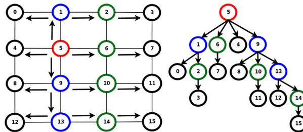
Fig. 4: Broadcast Tree: Static Routes Configuration
