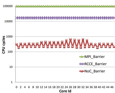
Fig. 27: Timing Results per Core for Barrier
