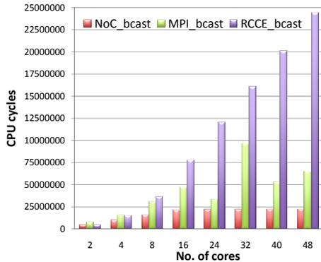
Fig. 26: Broadcast Timing over Cores
