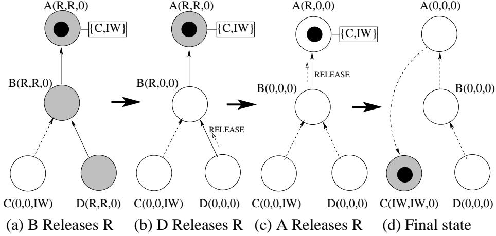
**Figure 5: Lock Release Example**
