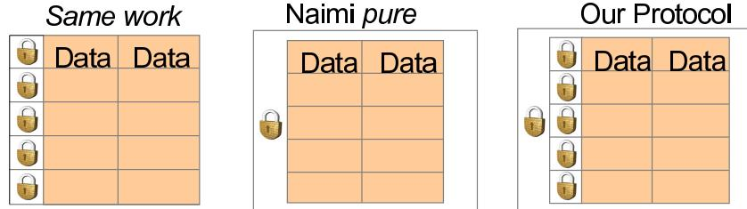
**Figure 11: Data Structures for Hierarchical and Non-hierarchical Locking**
