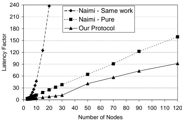
**Figure 13: Request Latency (as a factor of point-to-point latency)**
