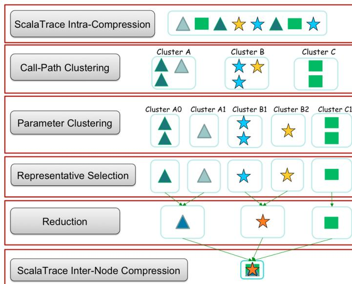
Figure 3: Overview of Proposed Clustering Algorithm
