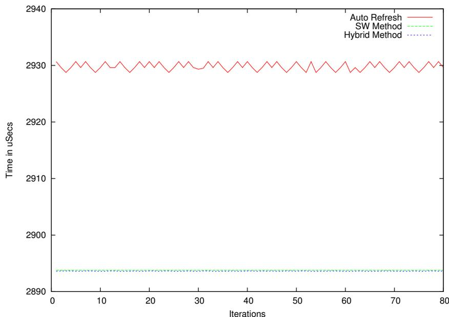
Fig. 8: Memory Latencies for DRAM Refresh Techniques on ARM Platform in Time Range [2,890-2,940]  $\mu$ s
