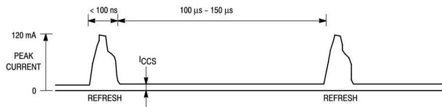
Fig. 2: Power supply current of a typical DRAM during refresh. See [15].
