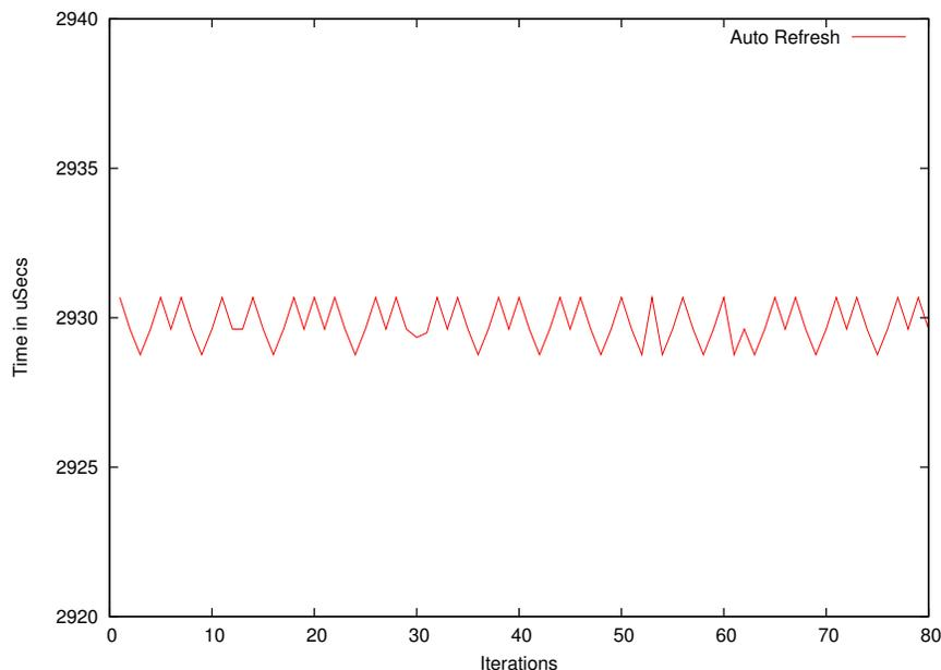
Fig. 6: Memory Latencies on ARM Platform using SDRAM. Time Range [2920-2940]  $\mu$ s. Software and Hybrid Values are so close that the Lines cover each other in the Graph.
