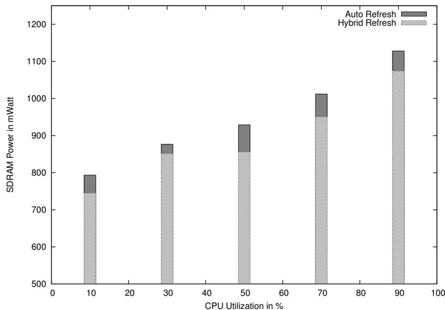
Fig. 9: Power comparison between different refresh methods under Linux. Range [500-1200] mWatt
