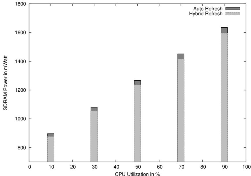
Fig. 10: Power comparison between different refresh methods under Micro C/OS-II. Range [700-1800] mWatt
