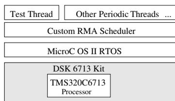
Fig. 3: System Architecture
