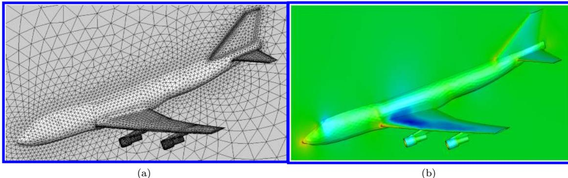
Figure 3: Transonic flow past a at a free-stream Mach number of  $M_\infty = 0.85$  and a angle of attack of  $\alpha = 2^\circ$ : (a) Unstructured mesh used for computation; (b) Computed pressure contours obtained by implicit rDG(P1P2)
