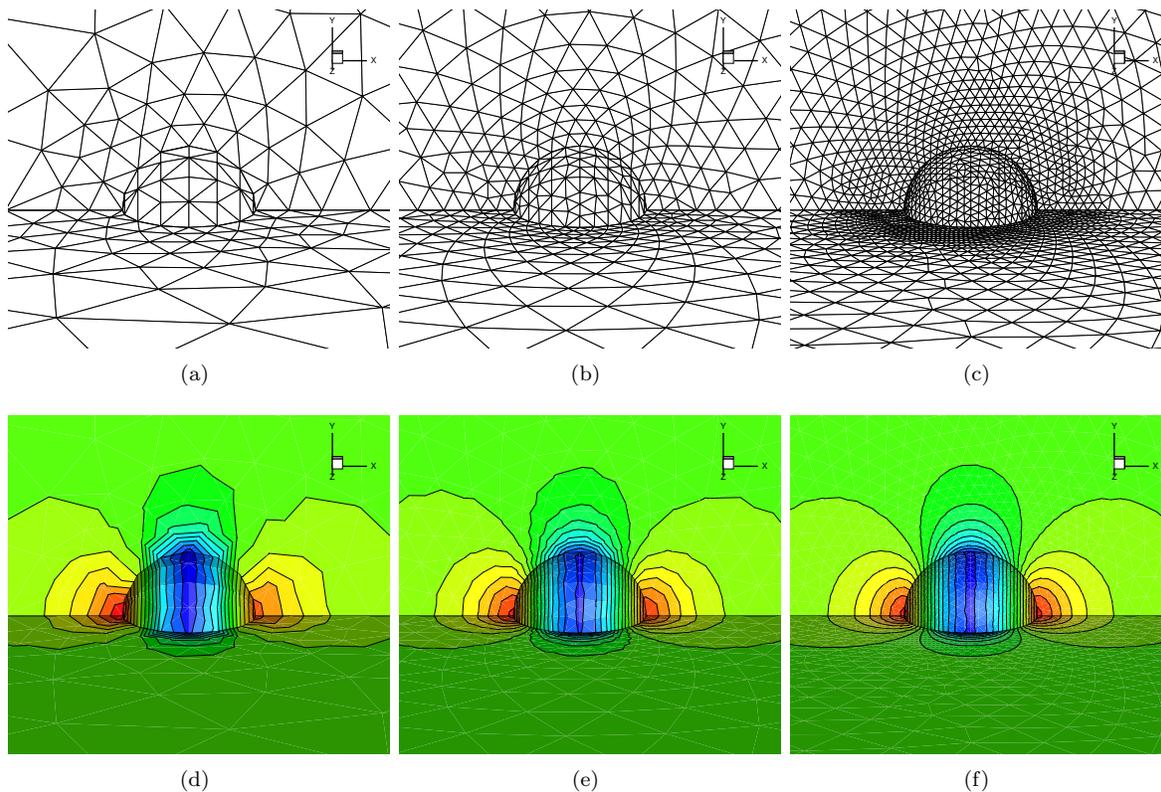
Figure 1: Subsonic flow past a sphere at a free-stream Mach number of  $M_\infty = 0.5$ : (a) – (c) Surface triangular meshes of the three successively refined tetrahedral grids; (d) – (f) Computed pressure contours obtained by implicit rDG(P1P2) on the surface meshes.
