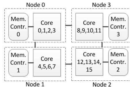
**Fig. 1.** 16 Cores, 4 Memory Controllers/Nodes
