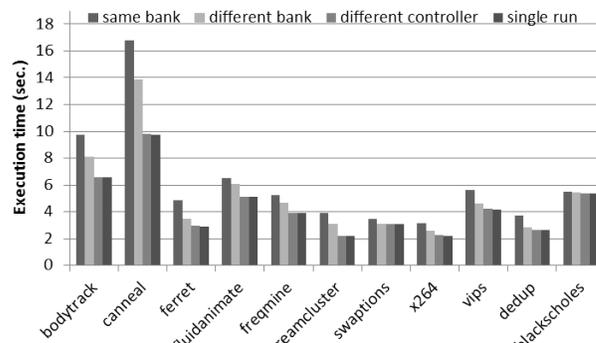
Fig. 4. Parsec: diff. controller/diff. bank/shared bank/single and 2.54% for ferret, are due to increased LLC contention for 4 tasks, which would be removed by LLC coloring.
