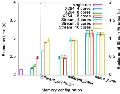
Fig. 5. Runtime of one X264 and 3/7/15 Stream Tasks
