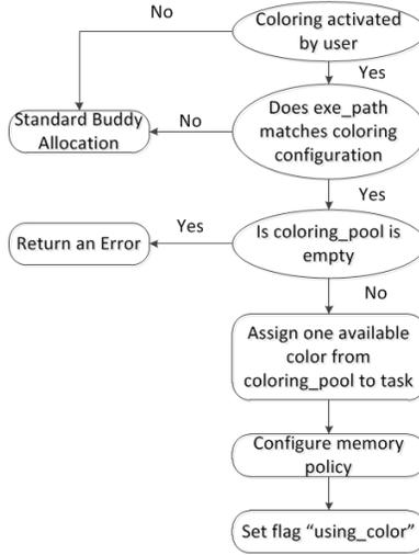
Fig. 2. Program Flow to configure memory coloring
