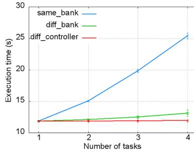
Fig. 6. Palloc: Avg. Memory Latency for Controller/Bank/no Coloring
