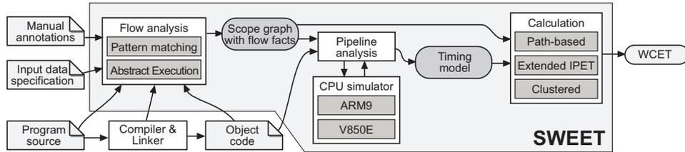
Fig. 8. Architecture of the SWEET timing-analysis tool
