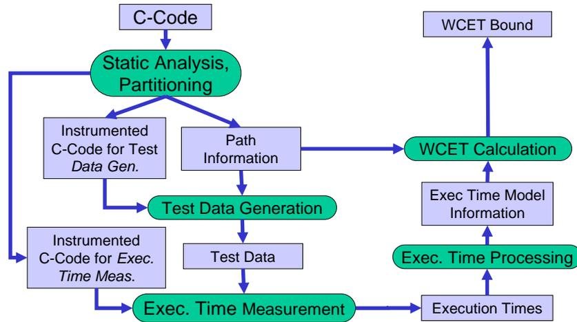
Fig. 7. Architecture of the TU-Vienna hybrid timing analysis tool
