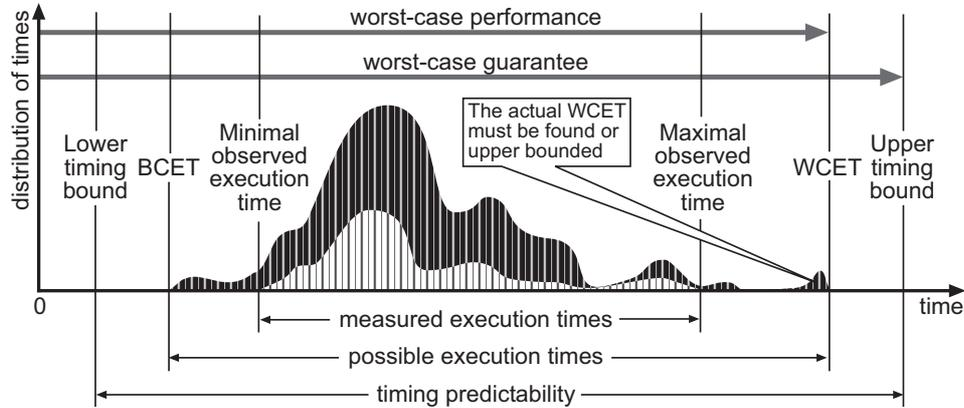
Fig. 1. Basic notions concerning timing analysis of systems. The lower curve represents a subset of measured executions. Its minimum and maximum are the *minimal observed execution times* and *maximal observed execution times*, resp. The darker curve, an envelope of the former, represents the times of all executions. Its minimum and maximum are the *best-case* and *worst-case execution times*, resp., abbreviated BCET and WCET.
