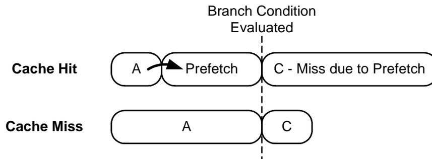
Fig. 2. A timing anomaly caused by speculation.
