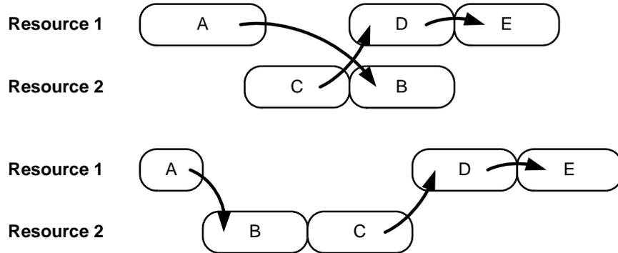
Fig. 3. A scheduling-caused timing anomaly.
