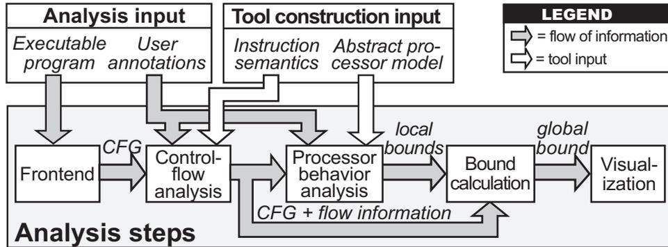
Fig. 4. Core components of a timing-analysis tool. The flow of information is shown by solid arrows. The dashed arrow represents tool-construction input.
