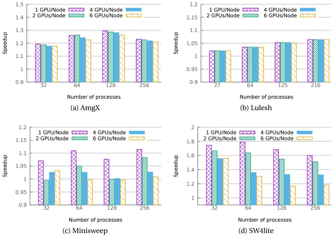
Figure 3.7: Predictions of speedup achieved in communication time when using GPUDirect over HostCopy for different applications (in strong scaling mode).
