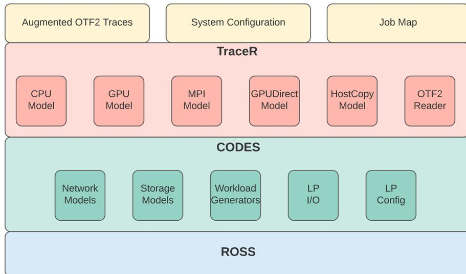
Figure 3.2: The TraceR-CODES simulation framework
