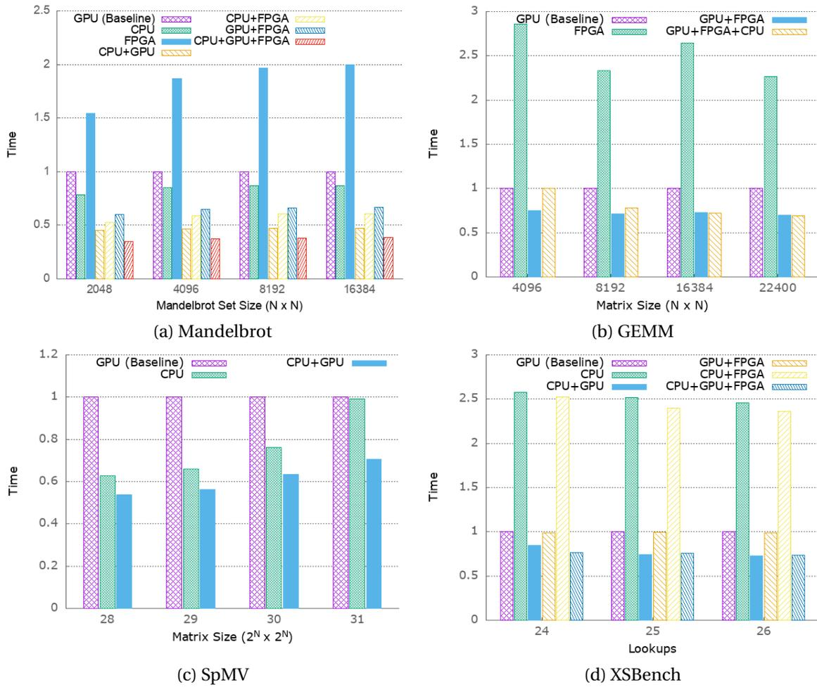
Figure 4.7: Normalized performance over various input sizes for various devices of each application.
