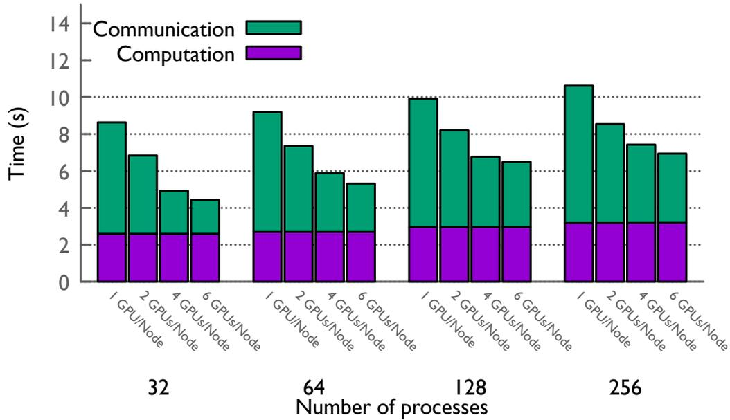
Figure 3.8: Minisweep communication/computation times for different node configurations while scaling the network bandwidth with number of GPUs/node.
