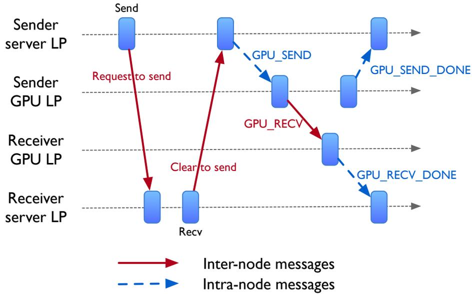
Figure 3.3: Timeline of GPUDirect messaging in TraceR-CODES.
