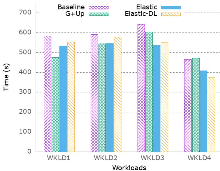
Figure 4.13: Overall workload time for the workloads with each of the scheduling algorithms
