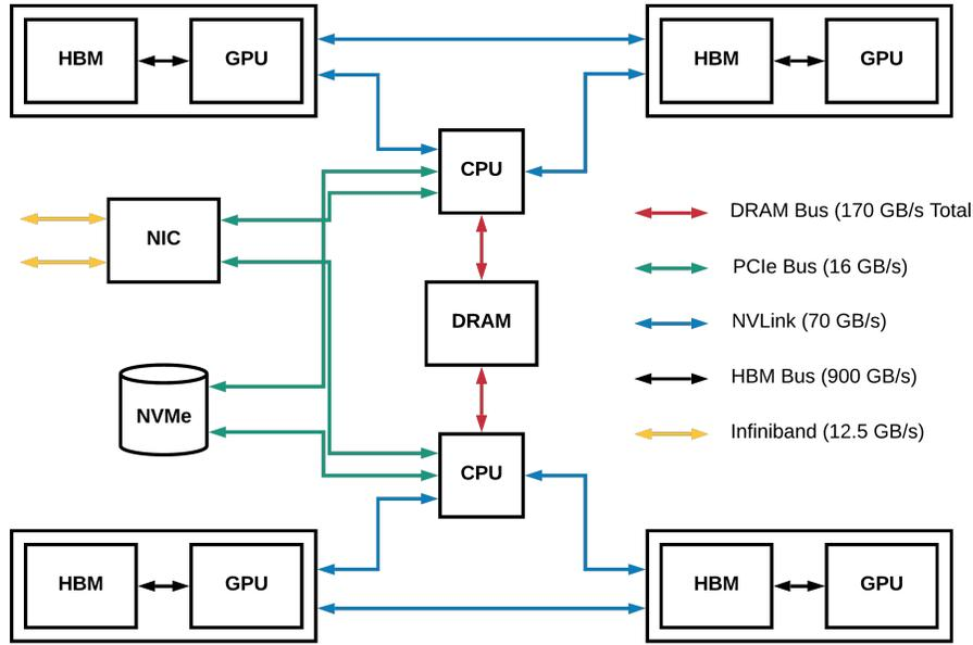
Figure 3.1: Organization of a compute node on the Sierra supercomputer at LLNL.
