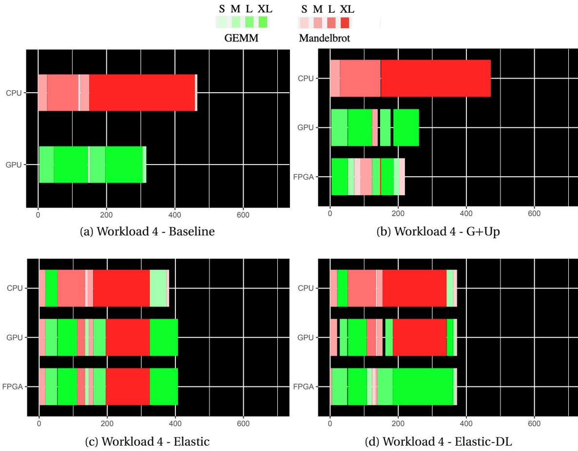
Figure 4.11: Timeline for the jobs on each accelerator in the two-application workload for each of the scheduling algorithms
