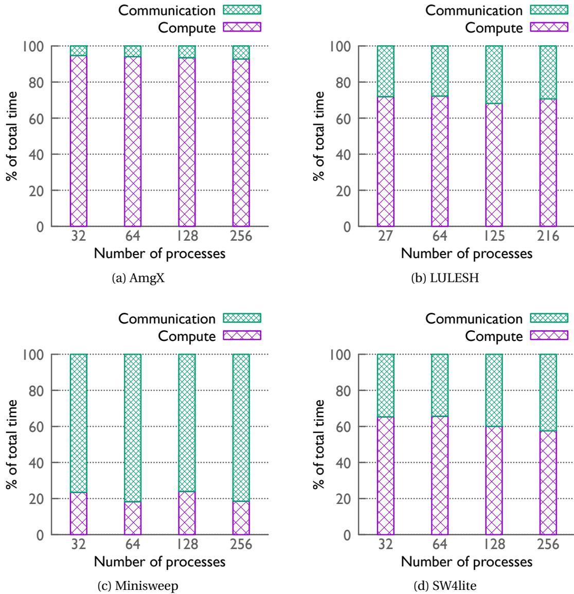
Figure 3.5: Time spent in computation versus communication (MPI routines) over different number of processes.
