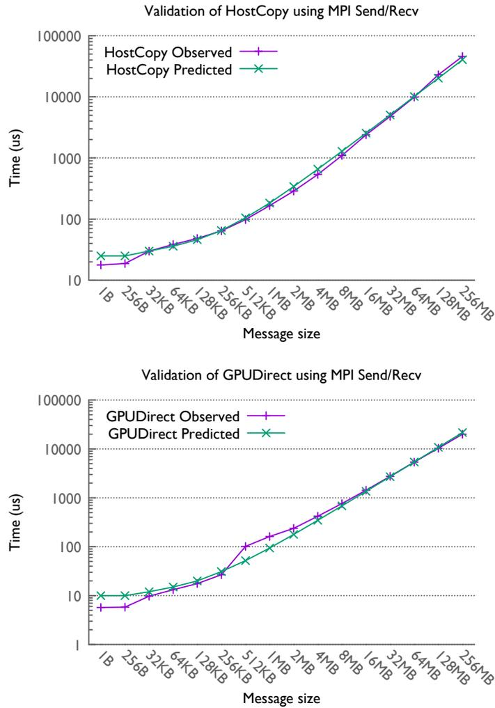
Figure 3.4: Plots showing the validation of HostCopy and GPUDirect simulations using TraceR-CODES.
