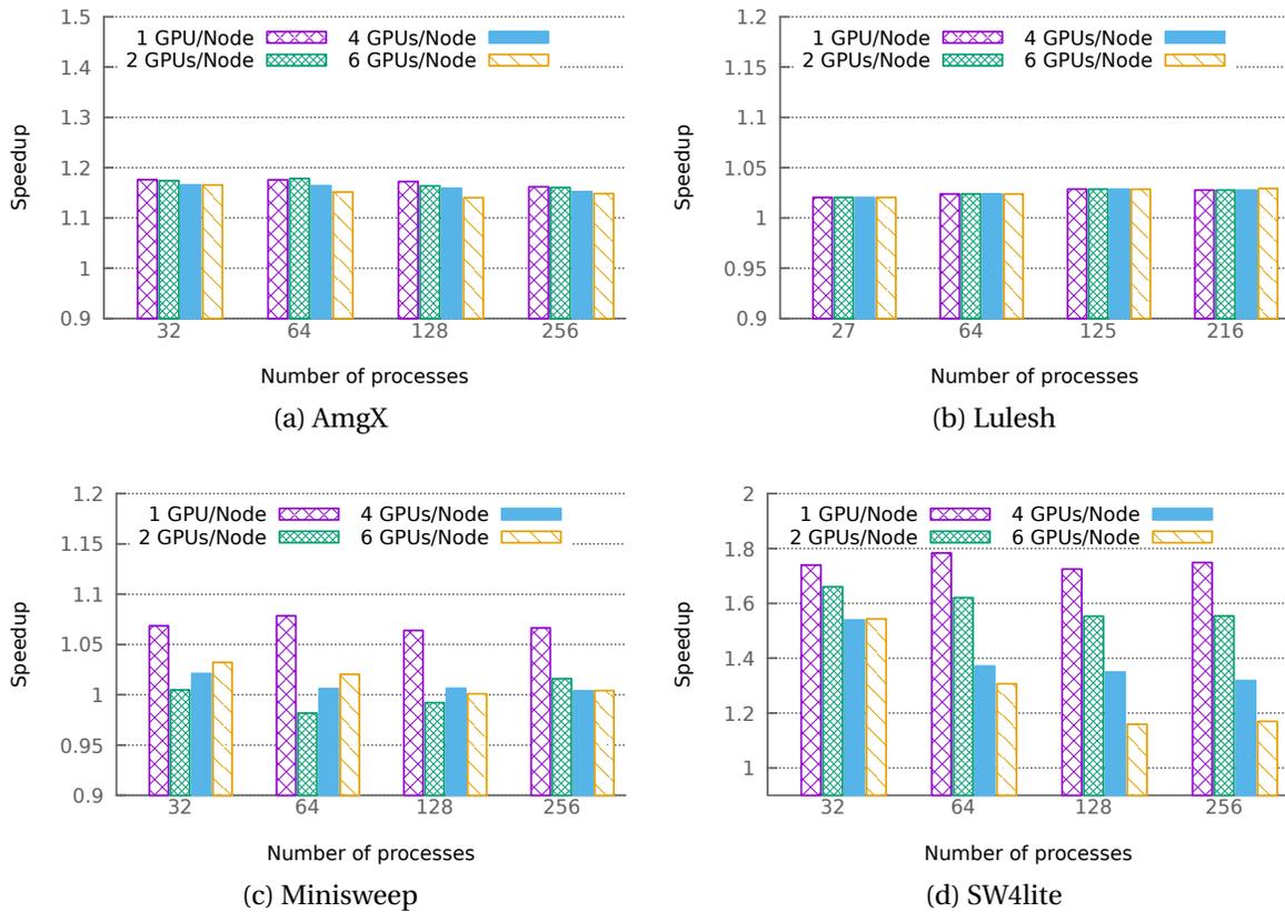
Figure 3.6: Predictions of speedup achieved in communication time when using GPUDirect over HostCopy for different applications (in weak scaling mode).
