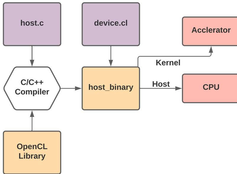
Figure 4.2: OpenCL application flow
