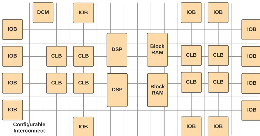
Figure 4.1: Block diagram of an FPGA with its components
