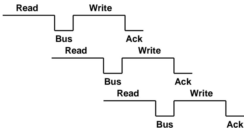
Since each subsequent request lags behind the previous request by  $D$  cycles, the last transaction starts  $((C_n - 1) \times D)$  cycles after the first push request is issued. The last transaction takes  $(2 \times B + D)$ . Thus, the migration delay incurred by SCMP is
