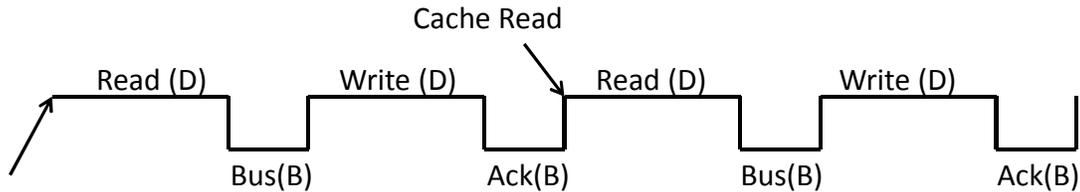
RCM in its current form is inefficient. Each cache read waits for the acknowledgment to arrive. When a cache is being read or written to, the bus is idle. When the bus is being accessed, the cache controllers are idle. To mitigate this under-utilization of cache and bus resources, we present our first novel scheme called Controlled Cache Migration Pipe-lining.
