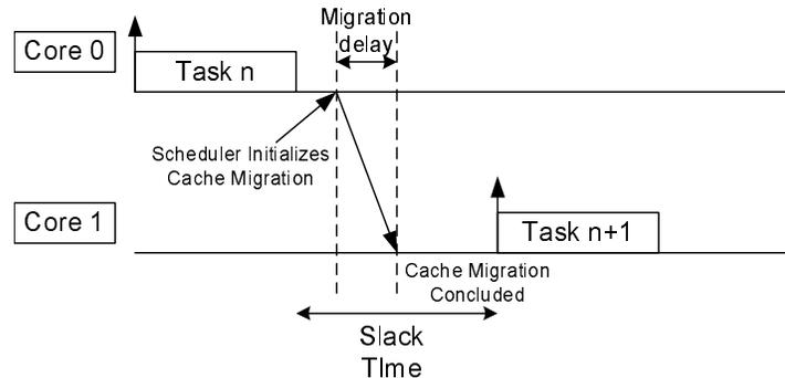
The simplest way of performing proactive cache migration is to unlock the lines at the source core. Thereafter, the target core can load and lock these lines. Both unlock and lock sequences can be encapsulated into threads spawned by the scheduler at the source and the target cores, in that order. Please note that this will contribute to the migration delay as shown in Figure 3.2. Such a scheme has following drawbacks:
