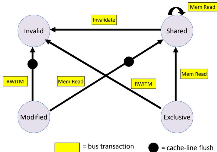
locally generated accesses. As we explained before, the snoop controller snoops the bus at every bus cycle for remote bus transactions. The following is a description of the state transitions caused by the snoop controller:
