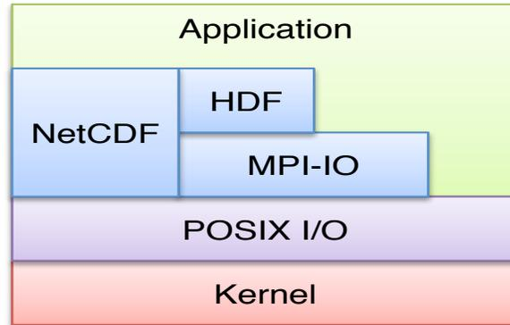
Figure 1.1: Typical Compute Node I/O Stack
