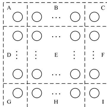
Figure 3.6: Distribution of Communication Groups of a 2D Stencil Code
