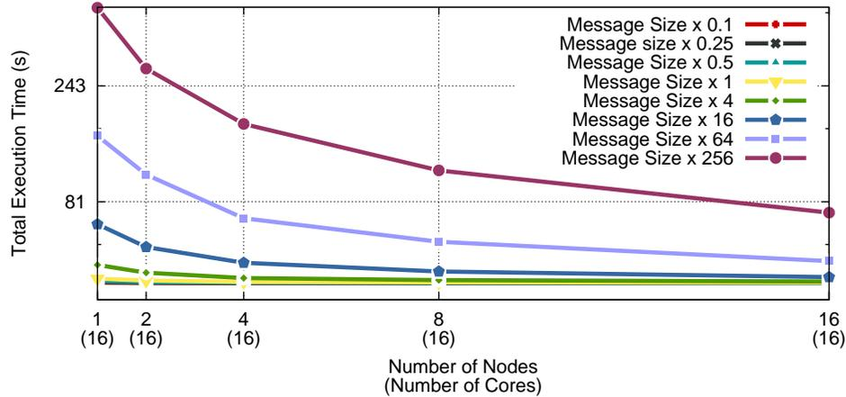
Figure 4.11: Impact of Communication Performance on BT
