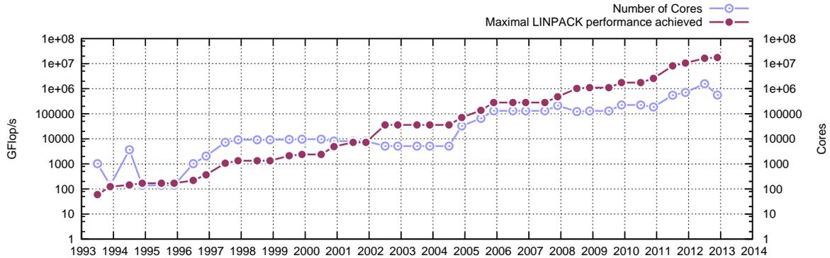
Figure 1.1: Performance Development of Supercomputers Since June 1993
