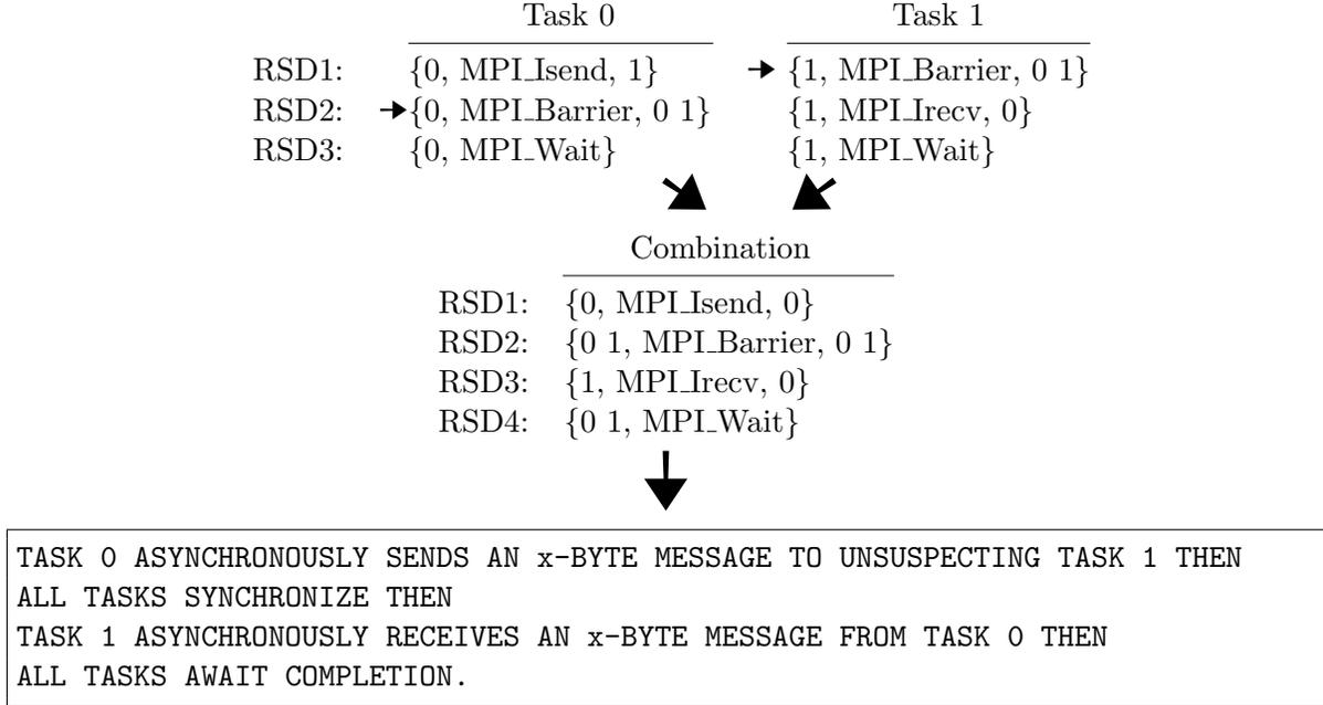
Figure 4.5: Operation of Algorithm 2
