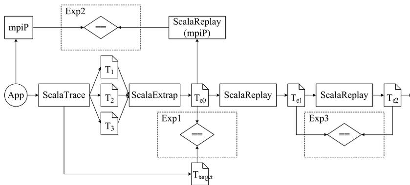
Figure 3.9: Correctness of Trace Extrapolation and Replay
