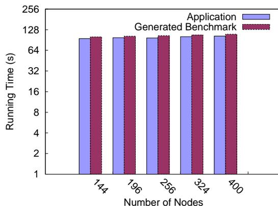
Figure 3.13: Timing Accuracy for the Extrapolated Benchmarks
