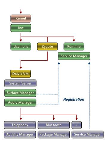
The bootloader loads the kernel and starts the init process
