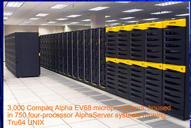
3,000 Compaq Alpha EV68 microprocessors, housed in 750 four-processor AlphaServer systems running Tru64 UNIX
